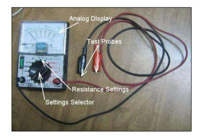
Shown in the figure is an Analog multimeter; it has a pointer moving on a panel like in an ammeter, or a voltmeter.
